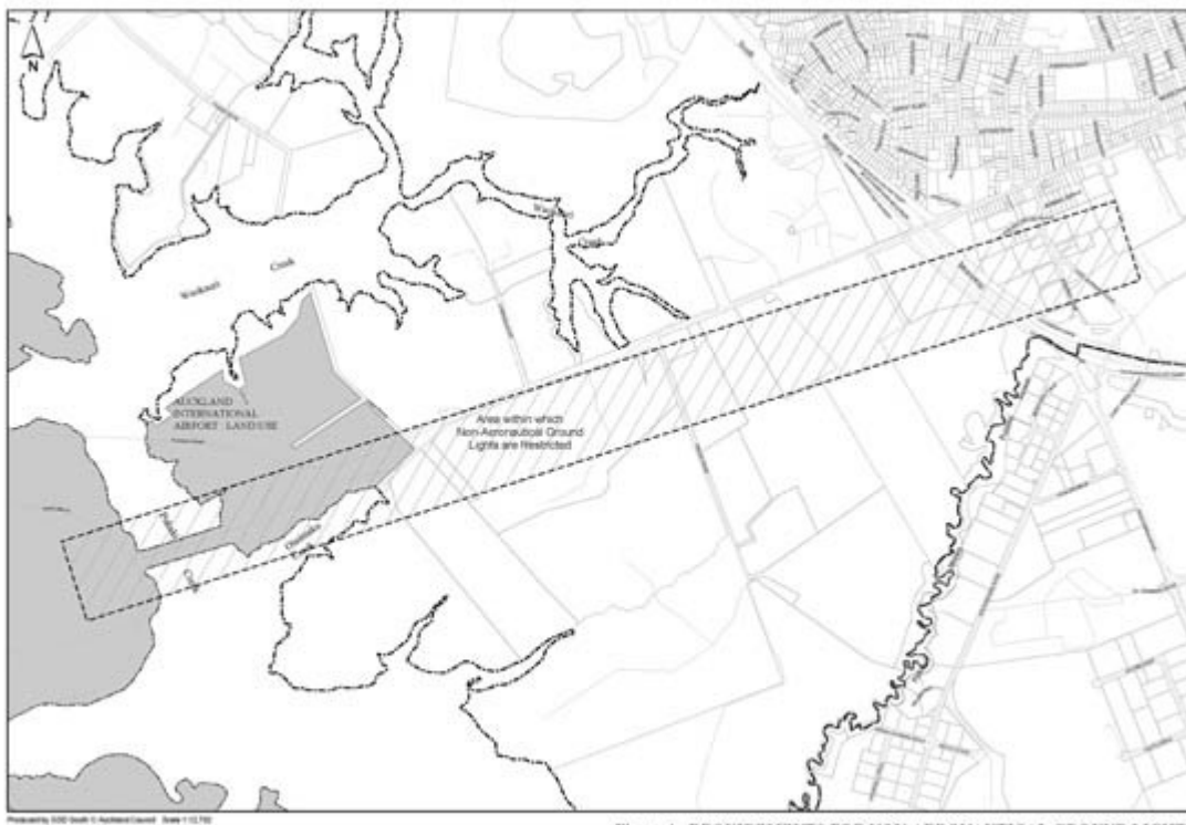
Figure 4 - REQUIREMENTS FOR NON-AERONAUTICAL GROUND LIGHTS APPENDIX 3
